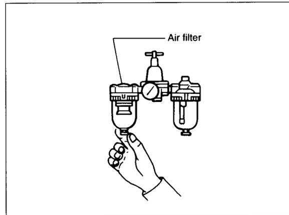
Check regularly to see if there is sufficient pneumatic oil in the oiler of the air set. Failure to maintain sufficient lubrication will cause O-rings to wear quickly.
